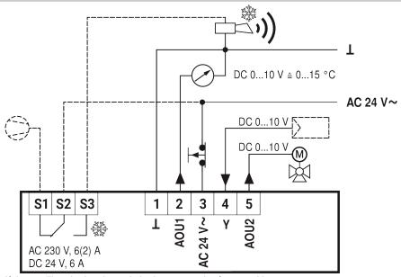
If the capillary leaks, the switch changes to the frost position. Min. active length material of capillary tube is 250 mm. Permissible cable length at 1.5 mm² diameter is max. 300 m.
