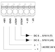
Connectors ST+ / ST- are only used for sensor types which additionally have a passive resistance sensor element for temperature measurement.
