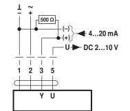
Control with 4...20 mA via external resistor
