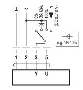
Control remotely 0...100% with Minimum limit with positioner SG..
