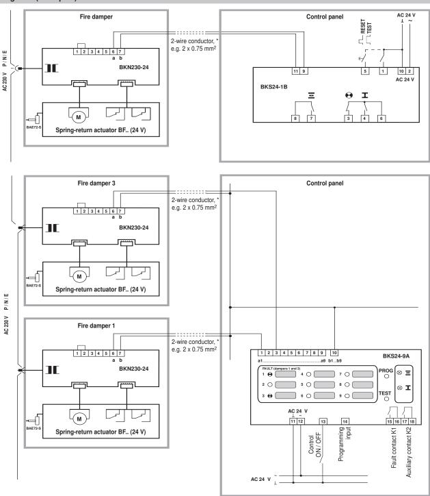
$<sup>^{\</sup>star}$  Lenghts of conductors: 2-wire conductors a/b max. 600 m (0.75 m²)
