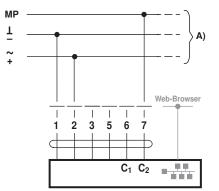
MP-Bus via 2-wire connection, local power supply
