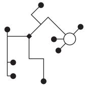
There are no restrictions for the network topology (star, ring, tree or mixed forms are permitted). Supply and communication in one and the same 3-wire cable • no shielding or twisting necessary • no terminating resistors required
