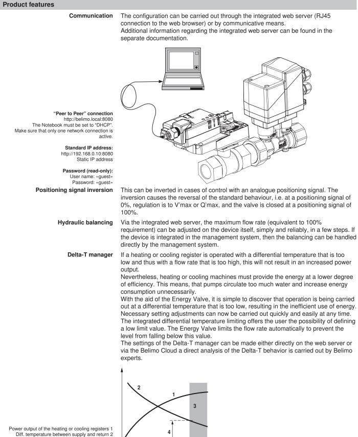
Diff. temperature between supply and return 2 Loss zone (heating or cooling register saturation) 3 Adjustable minimum differential temperature 4
