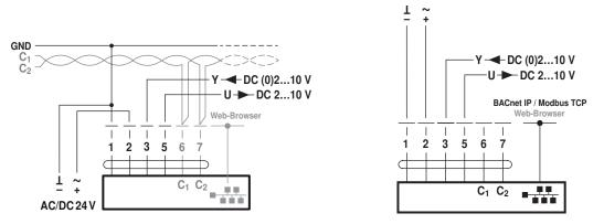
Override control and limiting with DC 24 V with relay contacts (with conventional control or hybrid mode)
