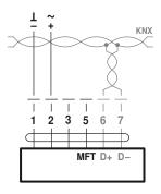
Signal assignment KNX: D+ = KNX+ (pink > red) D- = KNX- (grey > black) The connection to the KNX line should take place via WAGO connecting terminals 222/221.
