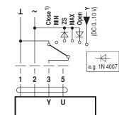
Override control and limiting with AC 24 V with rotary switch
