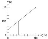
Control with 4...20 mA via external resistor
