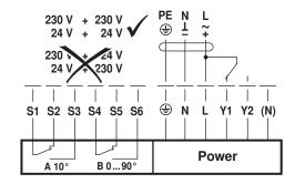
AC 24...240 V / DC 24...125 V, 3-point, Auxiliary switches
