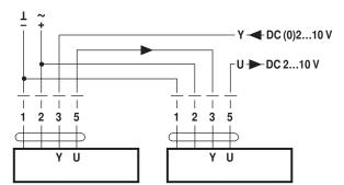
Control with 4...20 mA via external resistor
