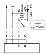
Control remotely 0...100% with Minimum limit with positioner SG.. positioner SG..
