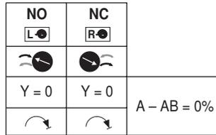
**Adaption and synchronisation** An adaption can be triggered manually by switching the direction of rotation switch from the left to the right twice within 5s or with the PC-Tool. Both mechanical end stops are detected during the adaption (entire setting range). Automatic synchronisation after actuating the direction of rotation switch once is programmed. The synchronisation is in the home position (0%).
